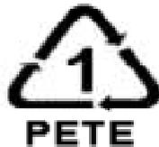
**Properties:** toughness, strength, heat resistance, barrier to moisture and gas. Density: 1.35-1.38 g/cc
